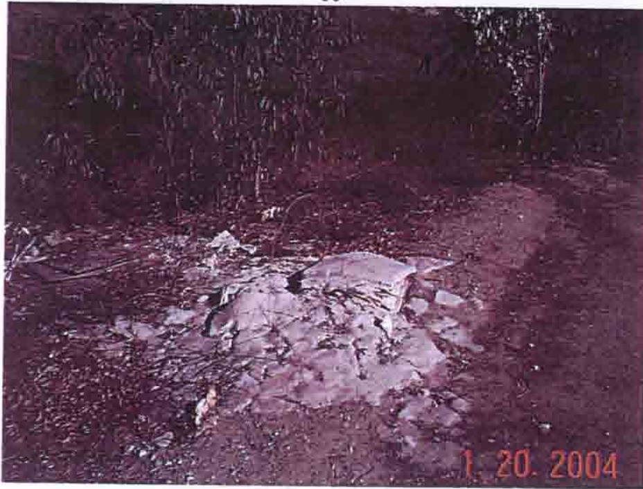
10. Construction debris in old railroad easement, possible asbestos-containing.
