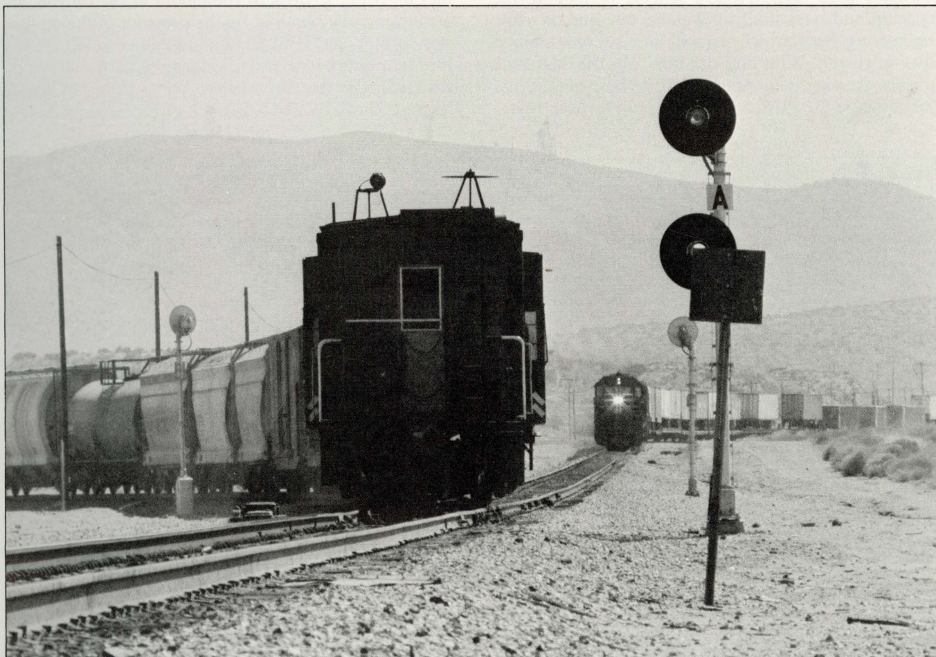
Headed to Colton via the cutoff line over Cajon Pass, an eastbound train is just clearing the switch at Palmdale as a westbound Saugus line local holds its ground on a 1.4% descending grade. —BRUCE KELLY
